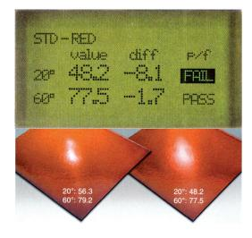
Paints, plastics and films all have different reflective properties. Metallic surfaces can reflect up to 20 times more light than non-metallic materials. With a measuring range of 0 to 2000 gloss units in the new micro-TRI-gloss you are prepared for almost anything.
