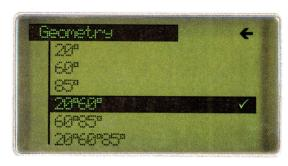
All selected geometries are measuring at the same location and the results are displayed instantly—including Difference, Pass/Fail and Statistics.
